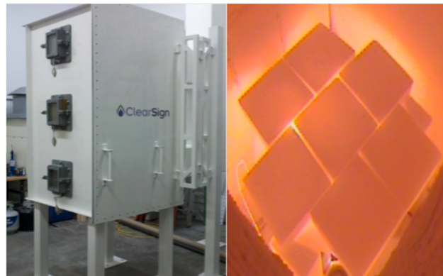
Figure 3: A process heater simulator fires natural gas at 2 MMBtu/hr. The right image shows a view of the Duplex surface in operation within the furnace as viewed by a high temperature camera.
