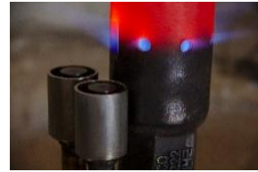
Figure 1 (Left) Top view of sensing probes (Right) Clearsign Eye pilot sensor shown mounted on operating pilot zoomed in at the pilot tip.
