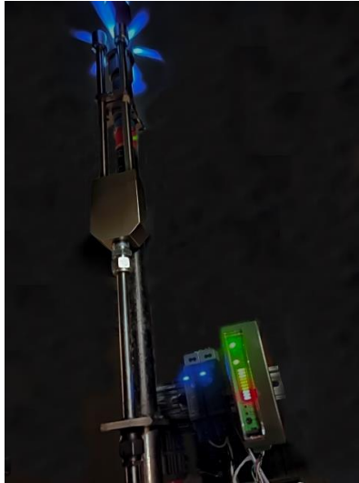
Figure 3 ClearSign Eye mounted on an operating pilot with the control unit shown on the far right mounted on a DIN rail next to the power supplies.
