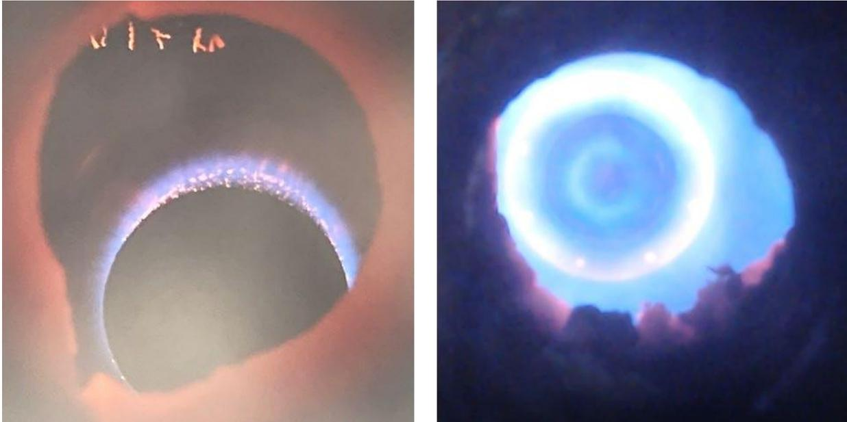
**Figure 13. Photographs of the burner flames – Baseline Mesh burner (left), ClearSign Core™-Rogue Burner (right)**
