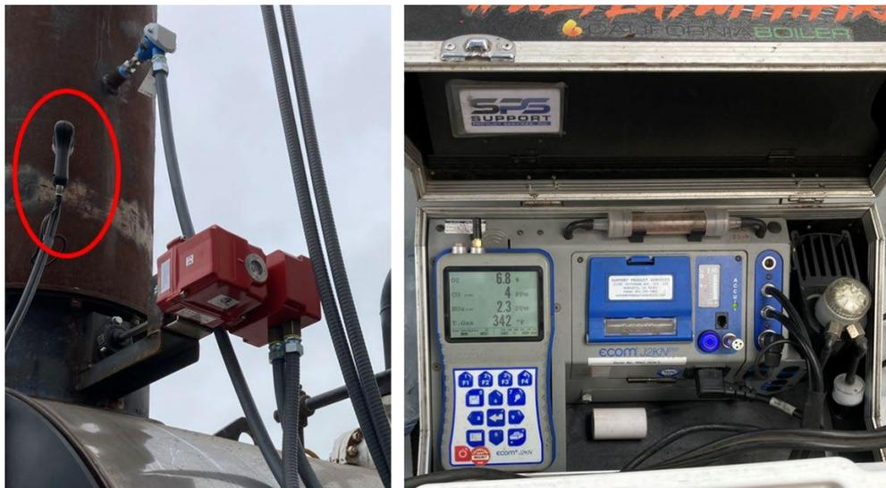
Figure 9. Emissions Probe Installed in the Stack (left), ECOM J2KN Analyzer (right)
