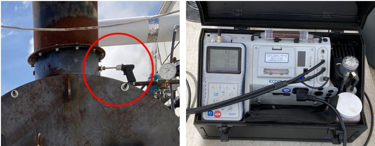
Figure 3. Emissions Probe installed in the Stack (left), and ECOM J2KN Analyzer (right)
