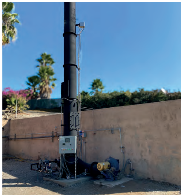
Figure 2. A ClearSign Core enclosed combustor. There is no visible light emission or smoke when in operation.
