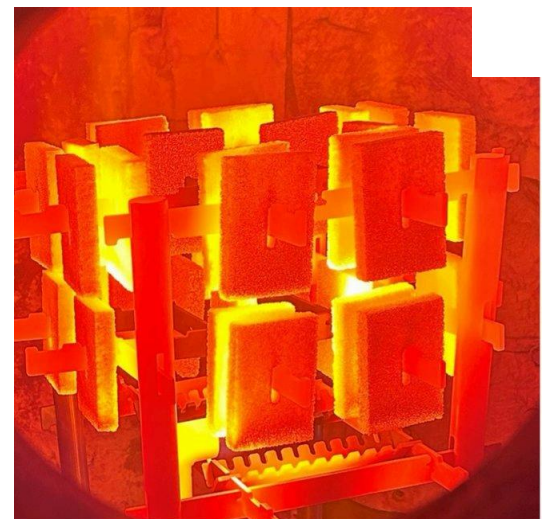
Figure 2 - ClearSign's Core Burner Technology operating with 100% hydrogen fuel.
